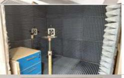
Anechoic EM Test Chamber
