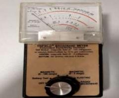
Trifield Meter Less EMF Inc. 30 Hz – 500 Hz Electric
