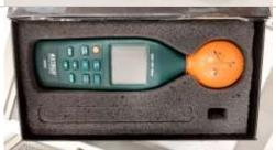
Radiation Hazard Meter EXTECH480846 10 MHz – 8 GHz
