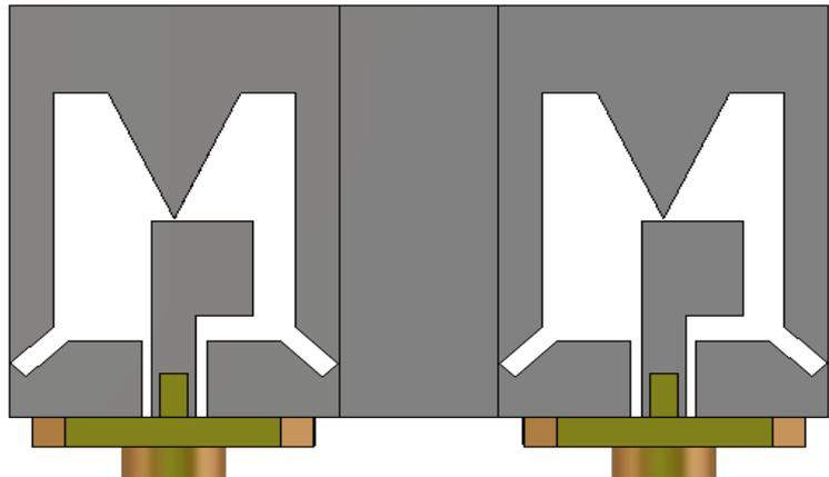
Geometry of the parallel two ports MIMO
