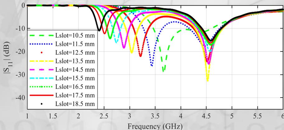
The antenna reflection coefficient in terms of the slot length ( $L_{slot}$ )
