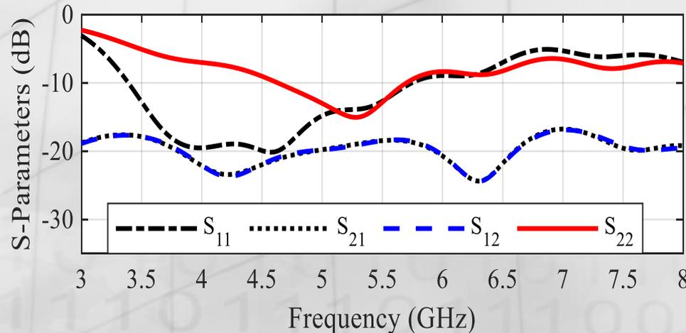
Simulated S-parameters of the polarized diversity dual elements MIMO antenna
