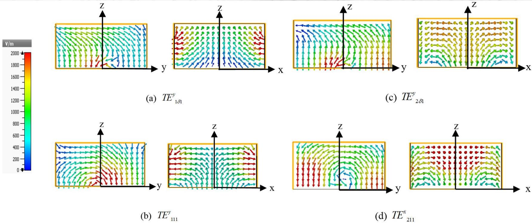
Simulated E-field distribution inside the proposed RDRA in both  $yoz$  and  $xoz$  planes at, (a) 3.5 GHz. (b) 4.1 GHz. (c) 4.8 GHz. (d) 5.2 GHz
