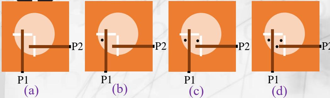
Geometry of various two ports CDR MIMO antennas, (a) Without vias, (b) With one via, (c) With two vias, and (d) With three vias
