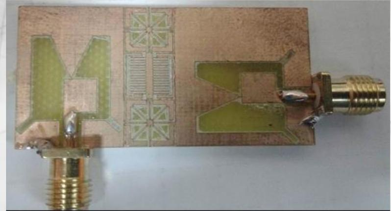
Geometry of the orthogonal two ports MIMO antenna with EBG
