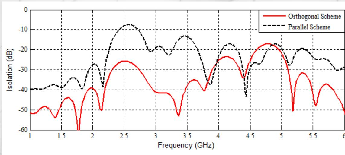
Isolation performance comparison between parallel and orthogonal schemes of MIMO DRA
