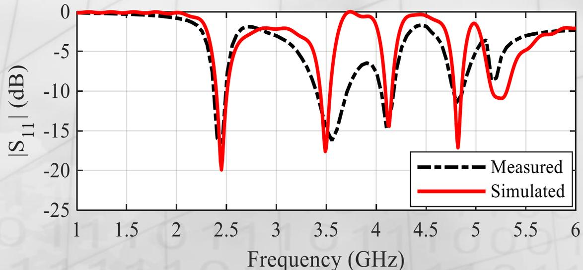
Simulated and measured reflection coefficient of the quintuple-band RDR
