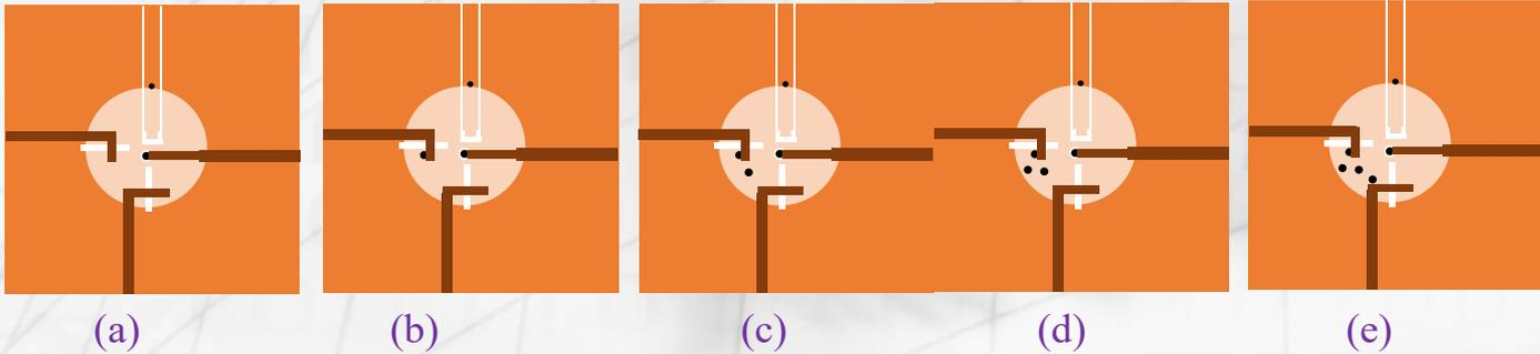
Geometry of various antennas used in the design procedure, (a) Without vias, (b) One via, (c) Two vias, (d) Three vias and (e) Four vias (Proposed antenna)
