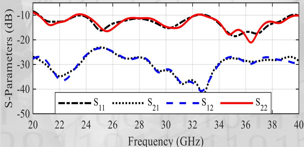
Simulated S-parameters of the parallel dual elements MIMO for the upper band
