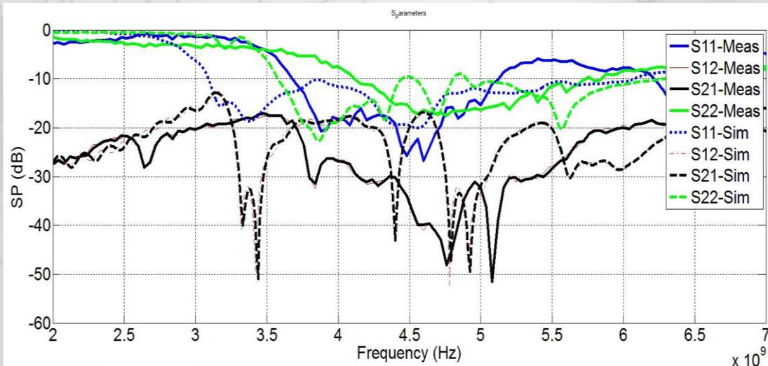
Simulated and measured S-parameters
