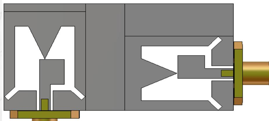
Geometry of the polarization diversity dual elements MIMO CPW slot antenna
