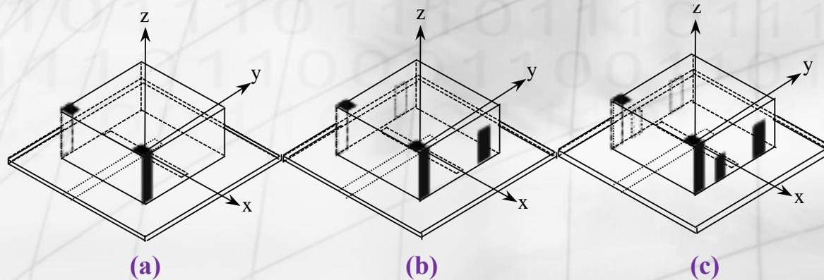
Geometry of various antennas used in the design procedure, (a) One VMSP, (b) Two VMSPs and (c) Three VMSPs (Proposed antenna)
