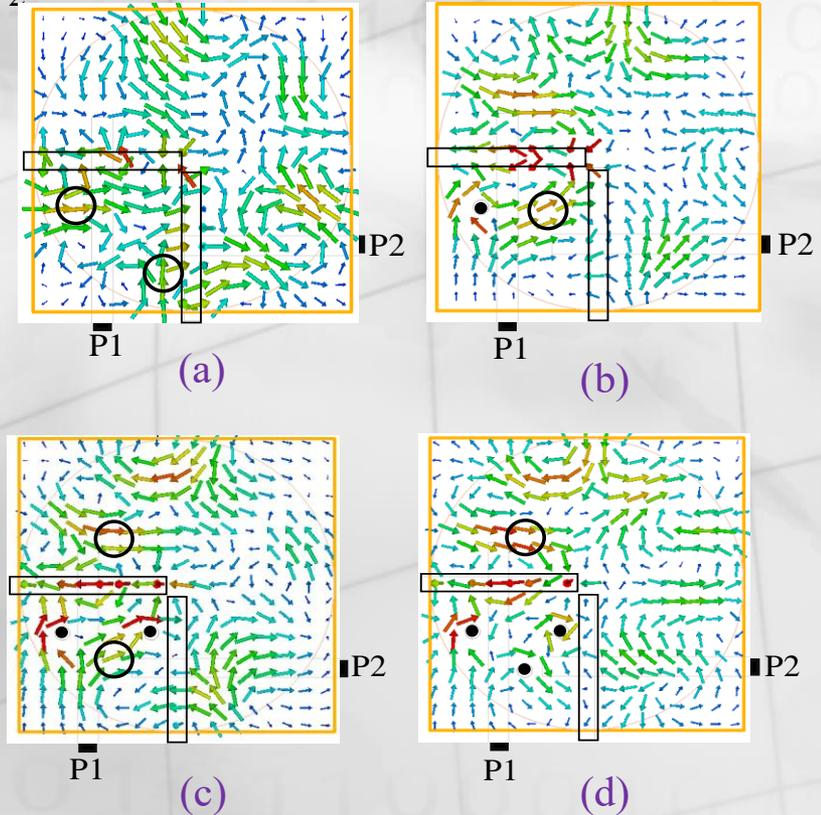
H-field distributions inside the two ports CDR MIMO at 8.8 GHz in the  $xy$ -plane for, (a) Without vias, (b) With one via, (c) With two vias, and (d) With three vias
