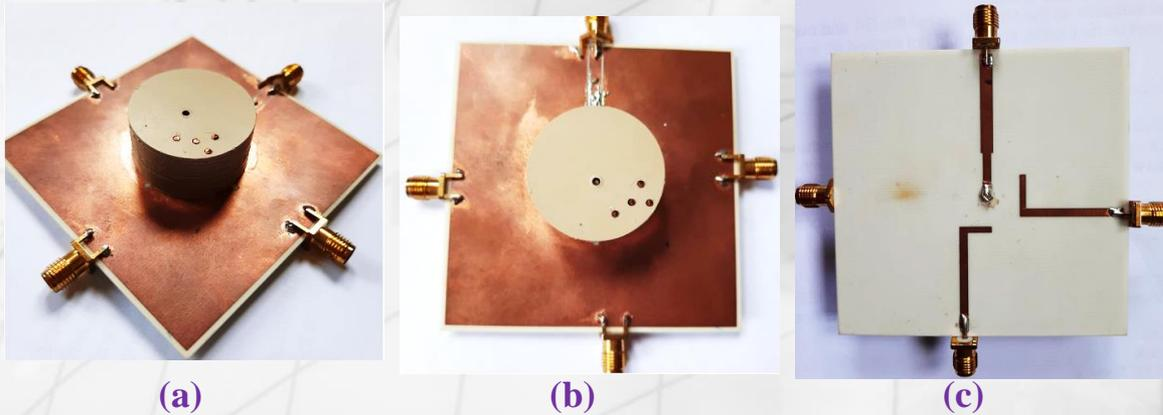
Fabrication of the proposed four ports single radiator CDRA MIMO. (a) 3D view, (c) Top view and (b) Bottom view
