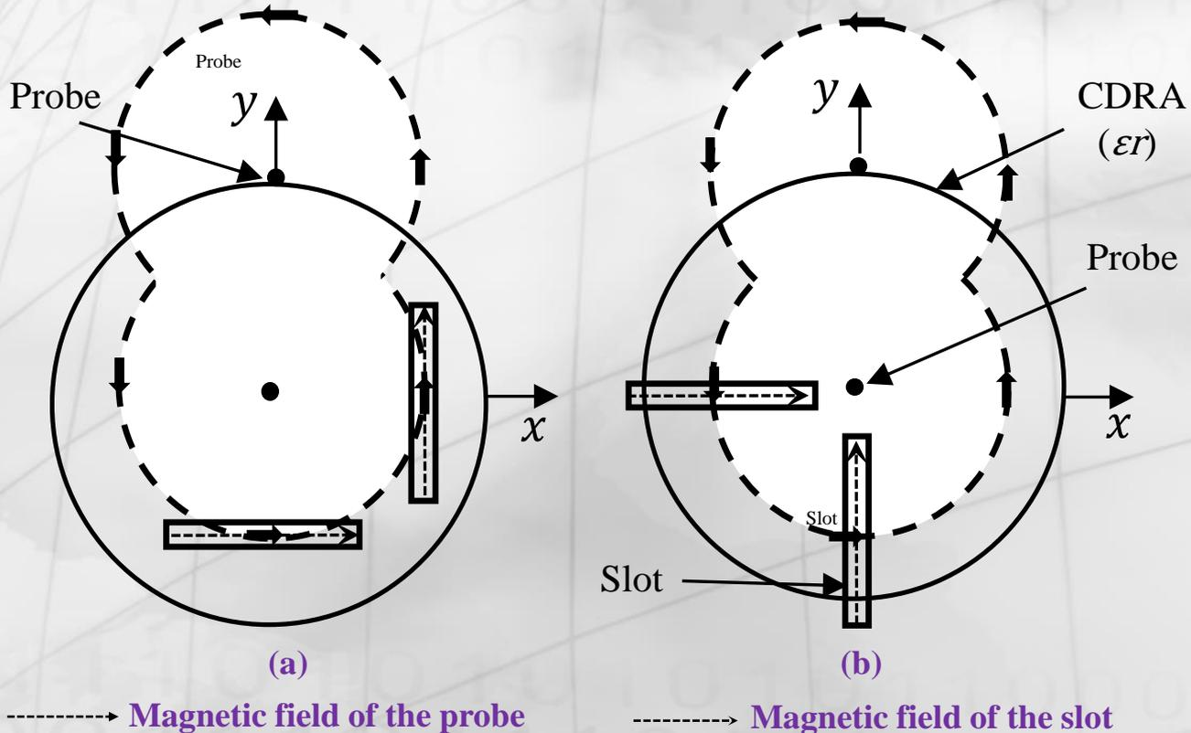
Magnetic fields of the probes and slots: (a) field probes align with the slots;
