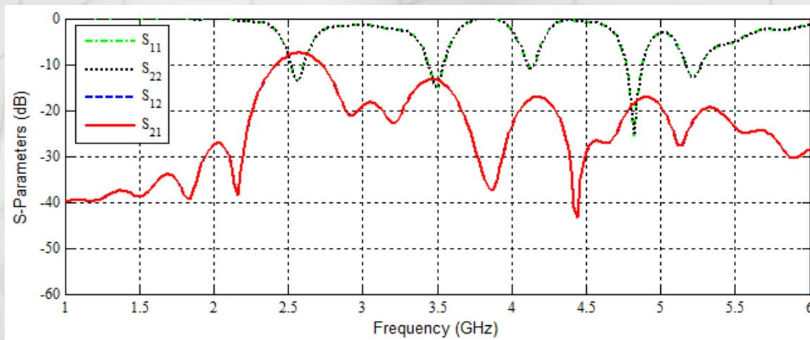
Simulated S-parameters of the parallel dual elements MIMO DRA
