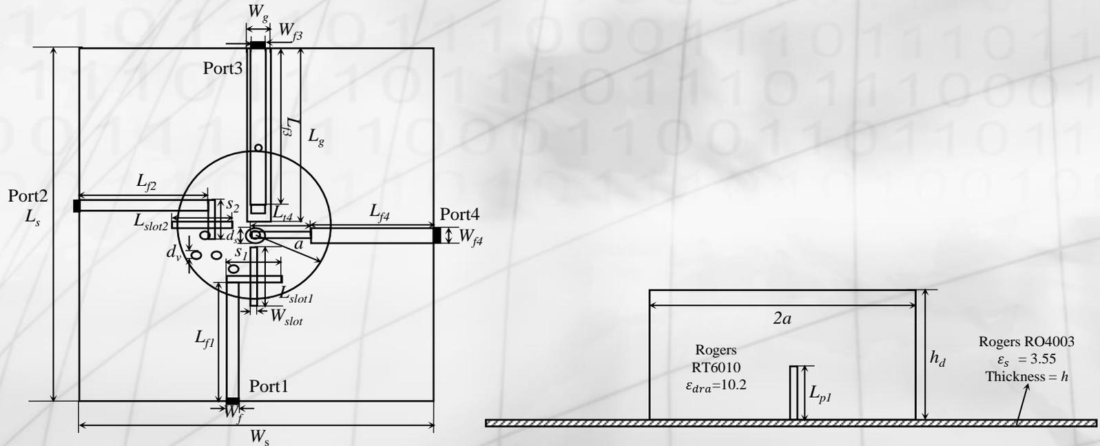
Geometry and dimensions of the proposed antenna top and side views
