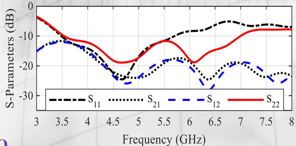
Simulated S-parameters of the parallel dual elements MIMO for the lower band
